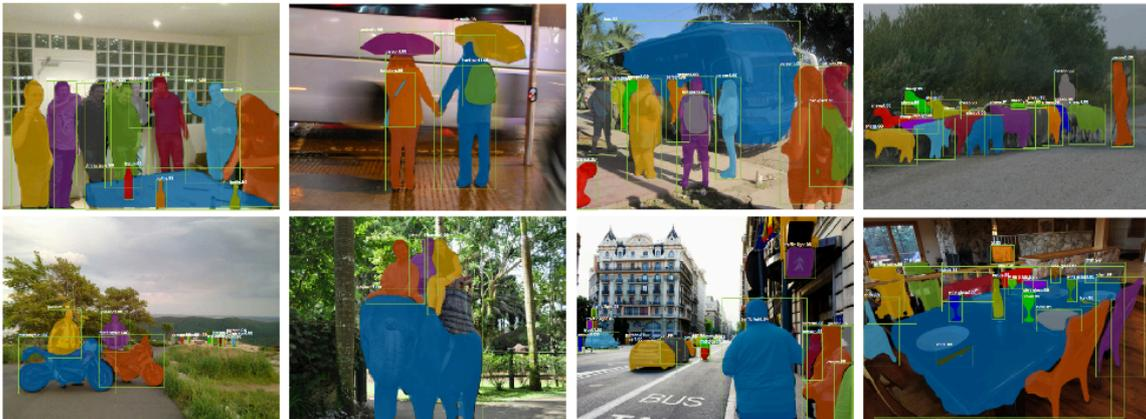
Figure 2. **Mask R-CNN** results on the COCO test set. These results are based on ResNet-101 [19], achieving a *mask AP* of 35.7 and running at 5 fps. Masks are shown in color, and bounding box, category, and confidences are also shown.
